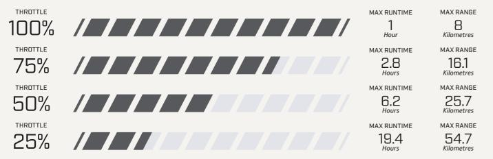
These figures are based on Mercury internal testing using a 13-foot Veer™ X13 boat (382-pound dry weight). Data derived from continuous use testing at designated throttle level on one full battery charge. Range and runtime may vary. Environmental conditions, boat type and load can influence performance.
